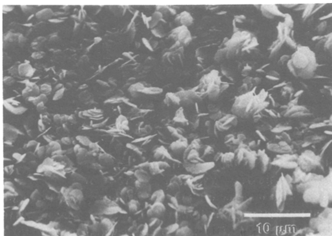
Fig. 2 SEM micrograph of PFHS-derived lead oxalate
